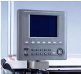
a simple monochromatic LCD monitor with an improved graphic interface for intuitive operation. The eye-level display offers improved ergonomics, while menu-interactive function buttons offer easy input and editing. The menu also features multi-lingual capability, available in 10 languages.
