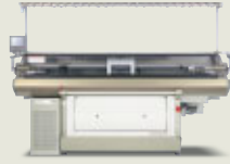
Computerized Flat Knitting Machine with Rib Transfer Capability
