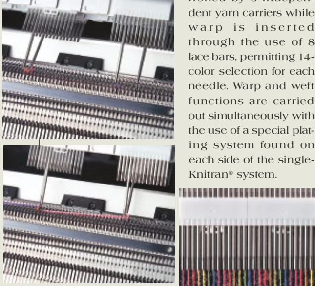
Warp insertion through the use of integrated lace bars.
