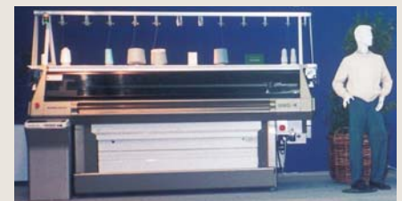
1995 Shima Seiki presents the SWG series, the world’s first fully-seamless computerized flat knitting machine, at the 12 th ITMA Exhibition in Milan, shocking the knitting industry.
