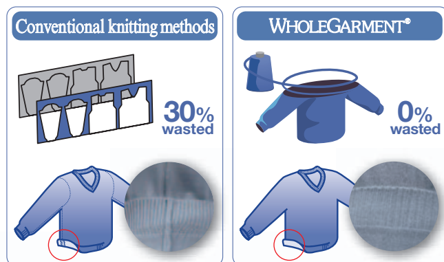
Conventional knitting methods cannot avoid the cutting loss and seam allowance in the course of cutting and sewing the parts
